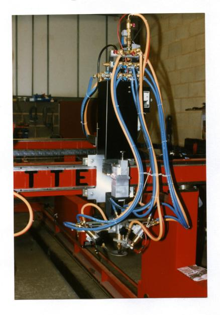
Advanced Cutting Systems manual indexing, Triple torch lightweight flame planing head complete with machine torches, gas control valves, mechanical height sensing device, and all necessary hoses for rectilinear plate edge preperation.
