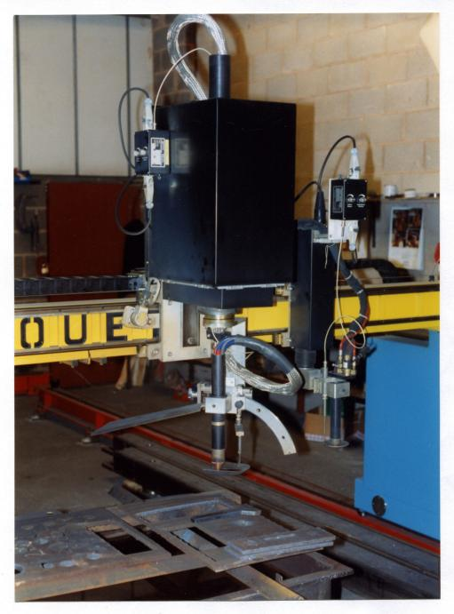
Advanced Cutting Systems single torch hole beveling head with motorised rotation through 365 deg and manual adjustment of bevel angle. Suitable for both Gas and Plasma applications. The torch head is supplied mounted onto a heavy duty motorised torch post.
