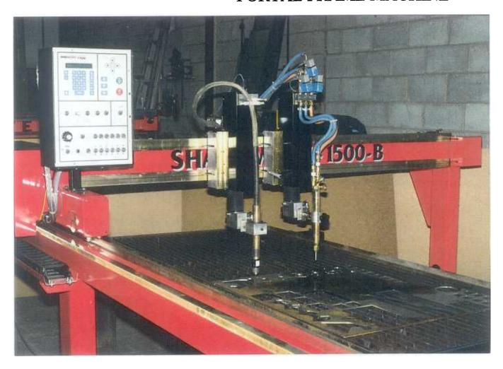
A dedicated CNC profile cutting machine for the smaller workshop, the Shadow portal frame system offers maximum productivity from a very compact work space. A choice of oxy-fuel gas or plasma torches makes the system ideal for the company with a mixed throughput of carbon steel and non-ferrous materials.
